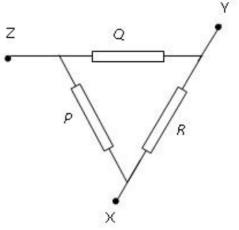
The diagram shows a circuit consisting of three identical resistors, P, Q, and R, each of resistance 4.0  $\Omega$  and connected as shown. If 3.0 A of current flows into point X in the circuit and 3.0 A flows out at point Y, then the power generated by resistor R is approximately ...
