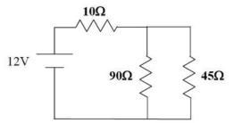
In the circuit above there is a current of 0.3 amps flowing through the 10 ohm resistor. How much current flows throught the 90 ohm resistor?
