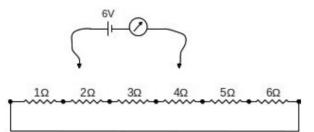
Consider six resistances connected as shown in the figure above. Note that the extreme ends are shorted. A circuit element consisting of a 6 V battery and an ideal ammeter can be connected across any two different points marked by dots in the resistance network. The *minimum* possible value of the current passing through tthe ammeter would be ...
